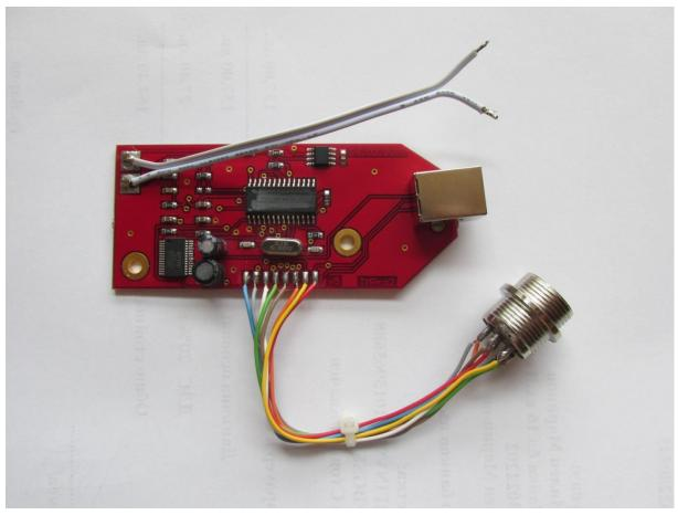
3.Solder pads of red antenna to antenna wires.It doesn`t matter which wire to which antenna pad will be soldered.
